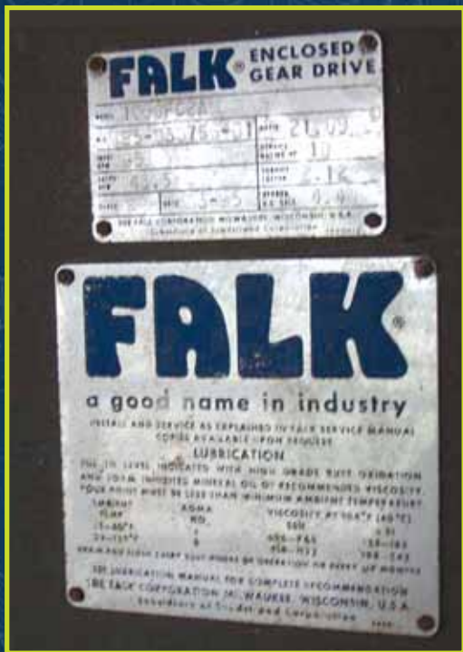
Figure 11. Gear drive faceplate label showing viscosity parameters
